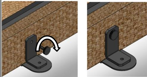
Turn the knob until the metal bracket is tight (This must be done on the side rail and center rail).
