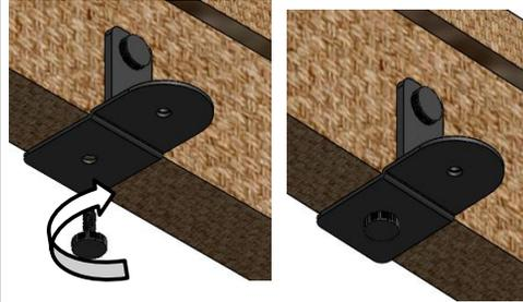
As in the upper part, in the lower part of the side a knob is also placed to hold the metal bracket (This must be done on the side rail and center rail).
