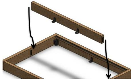
Line up each end of the center rail with the corresponding tapered slide connector and firmly push down into place, making sure the "up arrow" faces upward.
